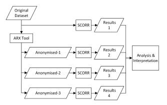
FIGURE 6. Test Setup for privacy metrics of original datasets.
