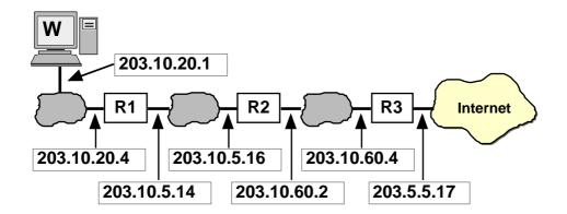
A user seated at the computer labelled W executes the traceroute command, with a destination address located somewhere in the "external" Internet. Give the list of IP addresses which will be revealed by execution of traceroute.
